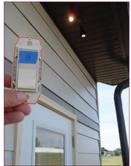
Photo 4 (left): Exterior view of the fresh air supply vent (lower) and exhaust air vent (upper) on the north side of the house. Note the specially designed downspout at the end of the house for rainwater harvesting from Equinox's steel roof. Photo 5 (right): Remote control switch used for zero wall penetration, exterior lighting circuits.
