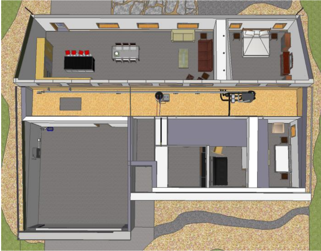
Figure 2 3D Sketchup view of Equinox House floor with corridor attic space shown. The CERV smart ventilator and HPWH are located in the corridor attic space.
