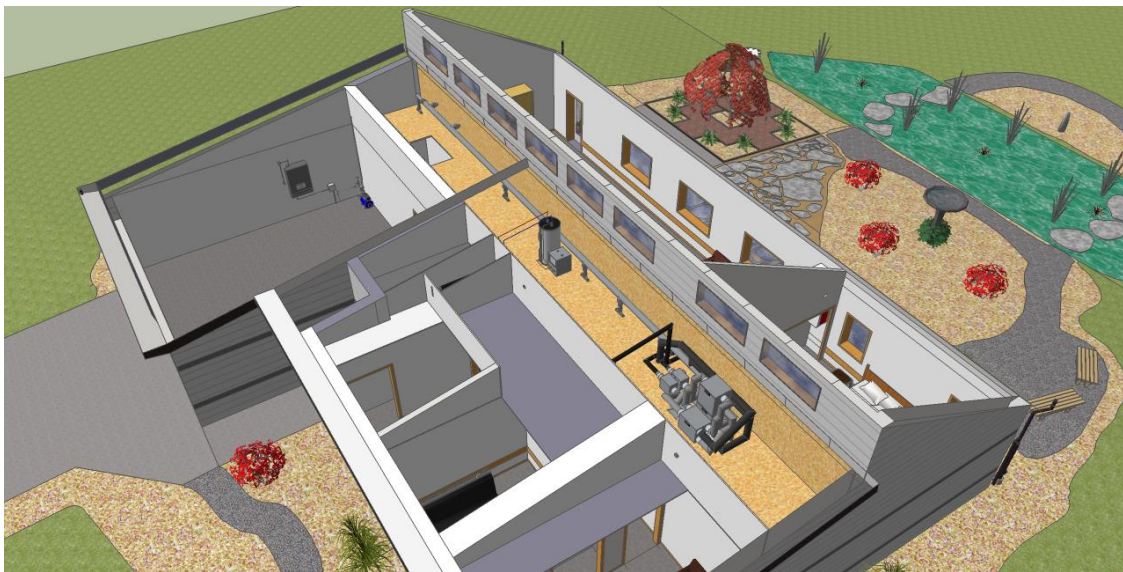
Figure 3 Roofless view of Equinox House showing additional detail of CERV ventilation ductwork. Fresh air is supplied to living room and bedrooms, and exhaust air is removed from kitchen, bathrooms (2 ½ baths) and laundry room.
