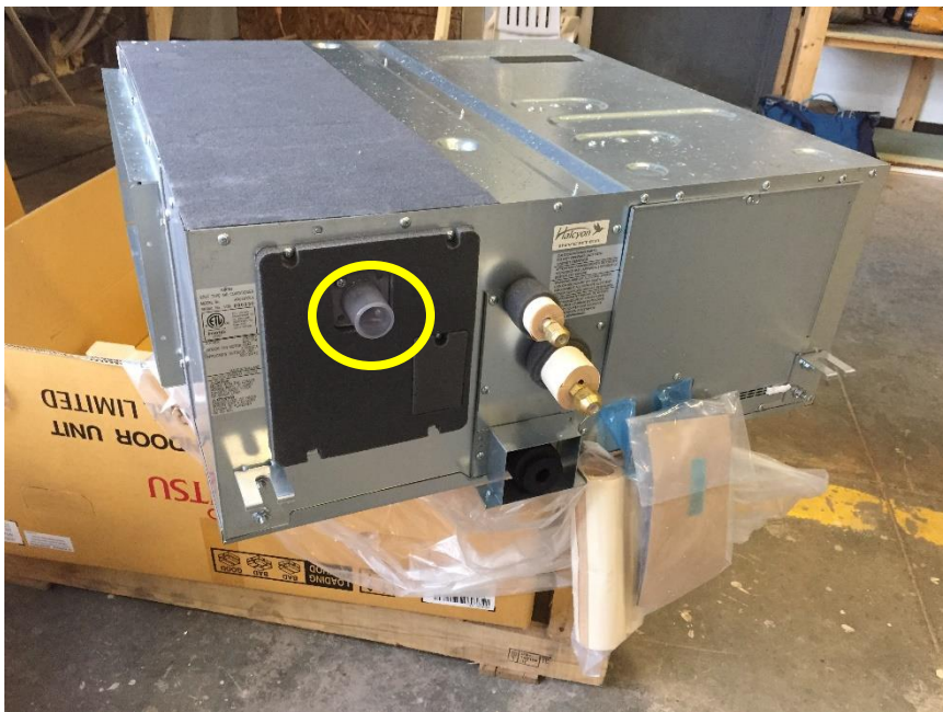
Figure 2 A “ducted” minisplit air conditioner indoor “head” can be concealed and connected to ductwork for air distribution. A circle is drawn around the condensate drain tube.
