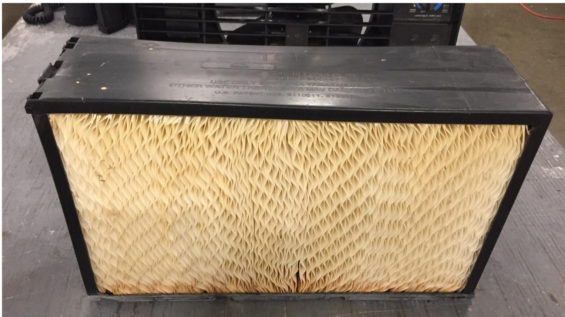
Figure 23 A fan blows air through a paper evaporator soaked in water.
