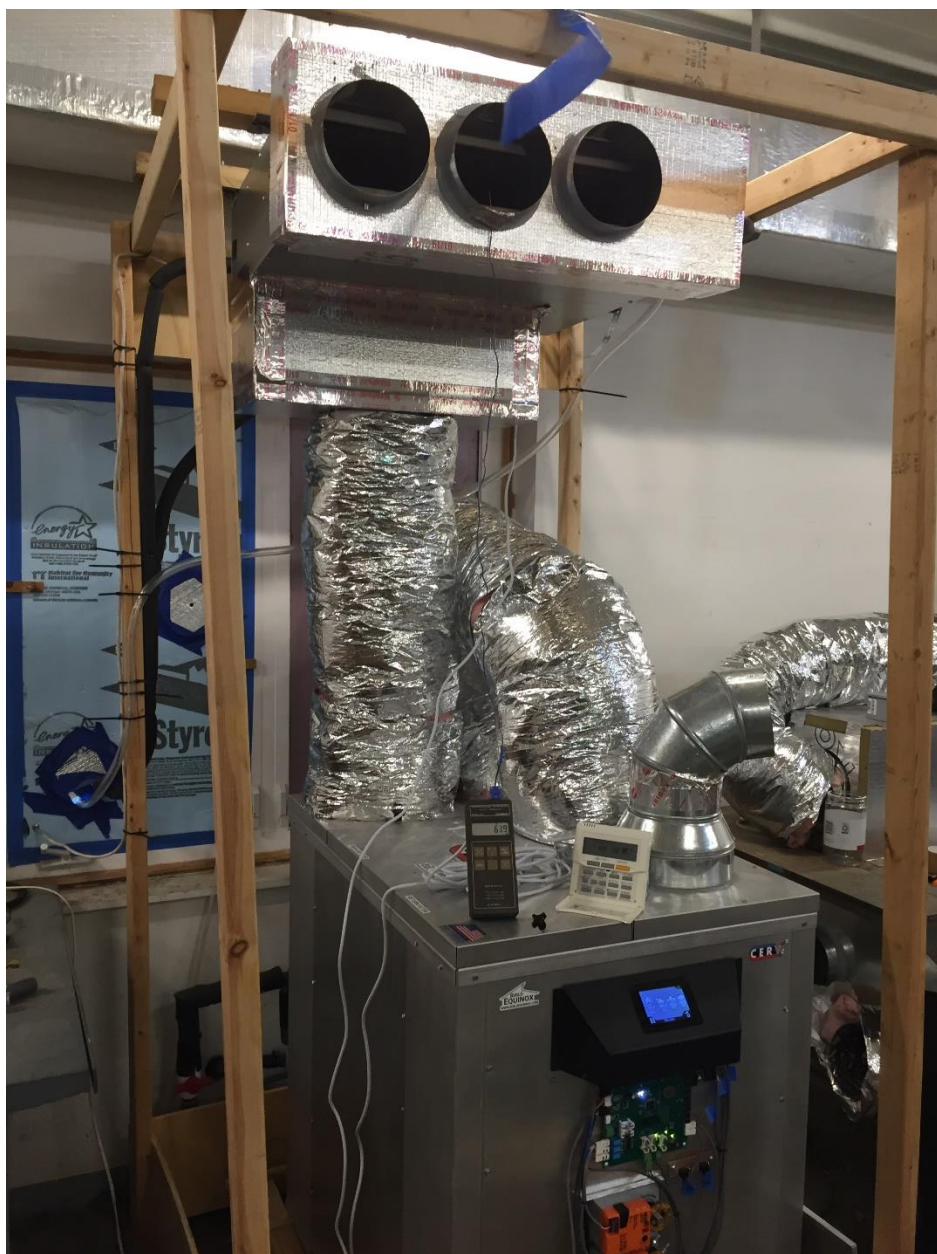
Figure 26 A CERV2 and high performance ducted minisplit heat pump are connected inline with an 8 inch diameter insulated duct at our Build Equinox laboratory. The CERV2 provides the brains for controlling the minisplit heat pump, seamlessly providing online control of automated air quality and comfort management.
