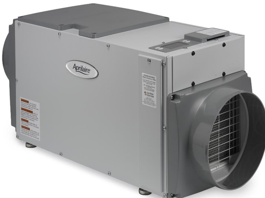
Figure 18 Duct mounted dehumidifier with 95ppd (45 kg per day) capacity operates with an airflow of 200 to 250cfm. This unit can be incorporated into the ductwork between a CERV2 smart ventilator and 1 ton ducted minisplit heat pump, with the CERV2 controlling all three units. Ducted dehumidifiers cost $1000 to $2000 depending on capacity and quality.
