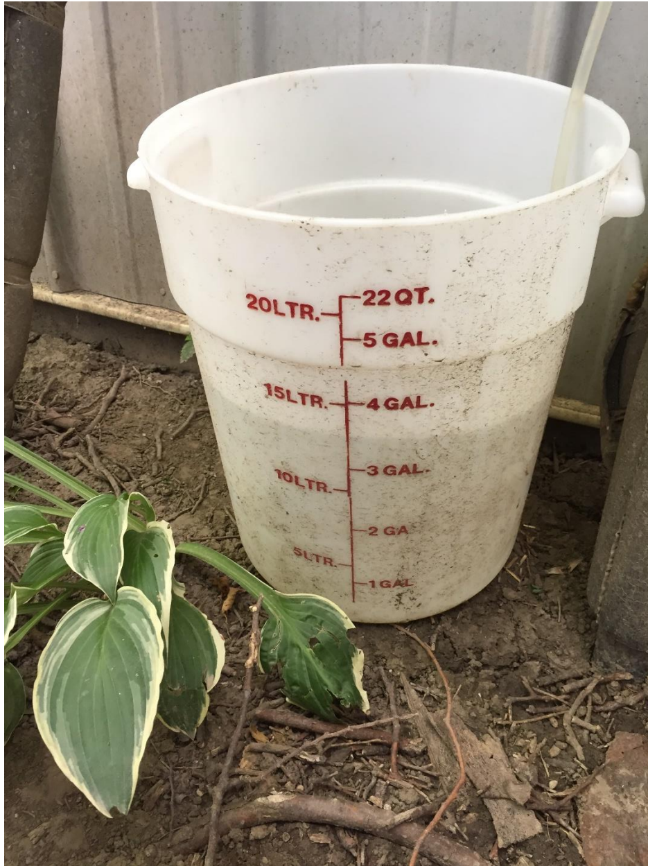
Figure 27 Condensation data is best collected manually coupled with daily logs of associated activities (cooking, showering, occupancy, weather extremes, etc). More than four years of collecting daily condensation data from Equinox House's heat pump, CERV, and HPWH required emptying 4000 containers of water!
