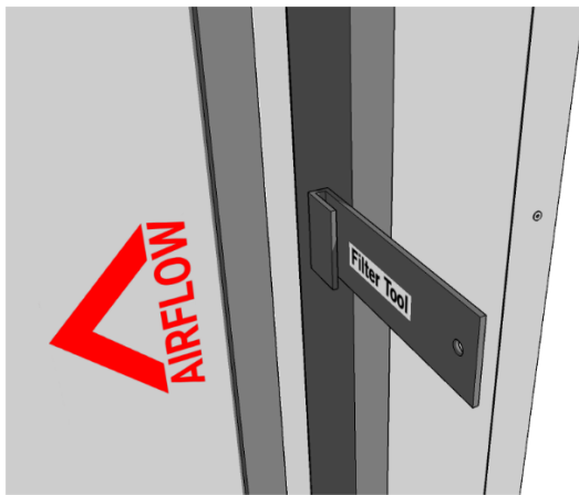
Insert supplied Filter Tool, hooking the old filter
