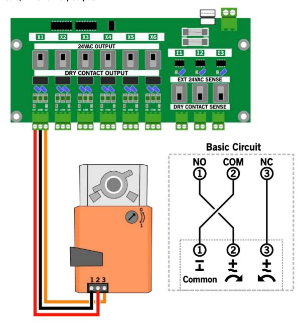
As opposed to the integrated XO Auxiliary output, the IO Expansion Board is capable of directly outputting 24VAC through its terminals without requiring connection to an external 24VAC source. NOTE: for this configuration, you must move the slide-switch above the terminal block towards the 24VAC OUTPUT label. LED indicators on the IO Expansion Board will light up above either the NO or NC terminals, to indicate which is active. Up to six zone dampers may be connected to the IO Expansion Board.
