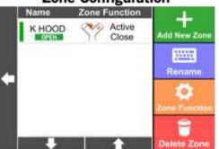
Create a zone with Active Close function. When zone is triggered, zone closes.
