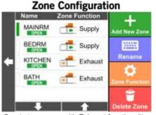
Create two zones with Exhaust functionality, and two with Supply.
