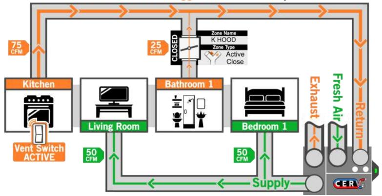
When the Wireless Ventilation Switch is activated, the Active Close damper in the bathroom return line closes down, reducing the airflow from 50 to 25 CFM, while the kitchen return is now favored, producing 75 CFM.
