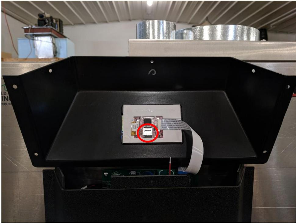
**Step 4:** While lightly pressing on the metal SD card housing, slide it down using a fingernail.
