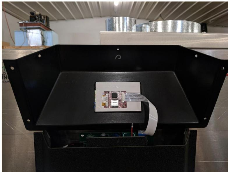
Rotate the top enclosure to see the circuit board on the underside (rotate the bottom towards you, top away from you). A ribbon cable connects the touchscreen to the main control board, and should be left in place. Take care not to bend or dislodge the ribbon cable from its connectors. The MicroSD card is located on the back of the screen held in place by a silver metal clip shown circled in red below.
