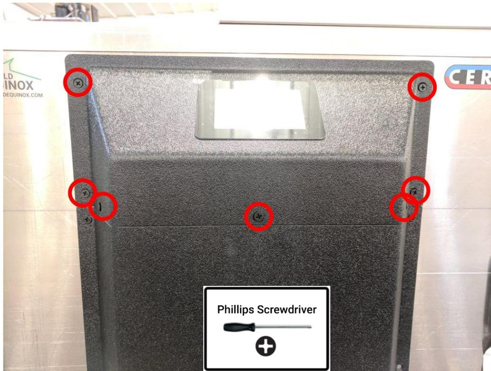
Locate the 7 black phillips head screws mounting the top touchscreen enclosure to the unit (shown below).
