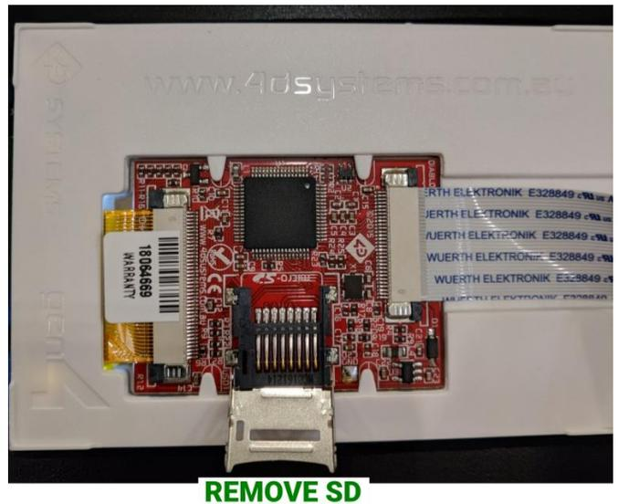
The metal SD Card housing should now flip down, allowing access to the MicroSD card.
