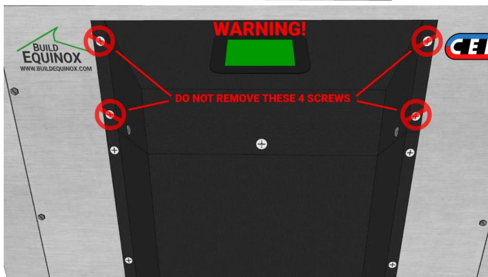
Once the lower front cover is off, the four screws for the lower access panel can be removed. Screw locations are shown below. With the screws removed, the panel will be free to come out.
