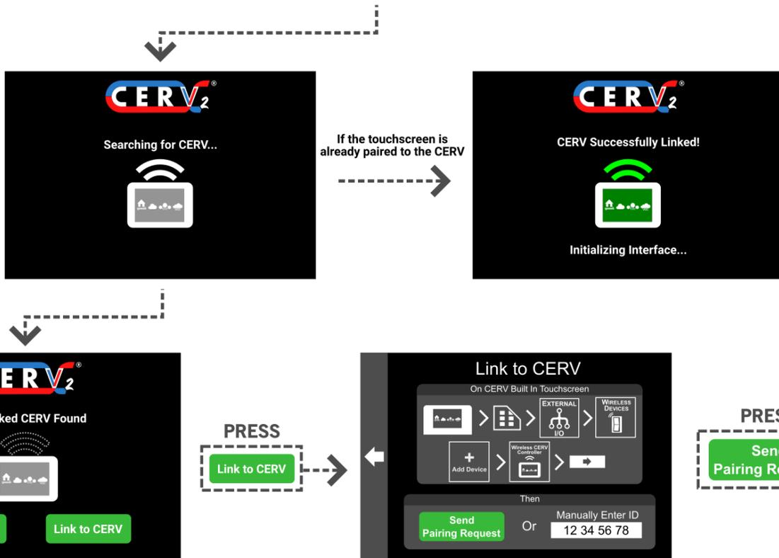
After reaching the Link to CERV screen, the base CERV must be put into pairing mode so the two can be linked together. Follow the instructions on the next screen to navigate to the correct screen on the base CERV. The touchscreen may be paired by either pressing the green Send Pairing Request button, or manually entering the wireless touchscreen's wireless touchscreen ID.
