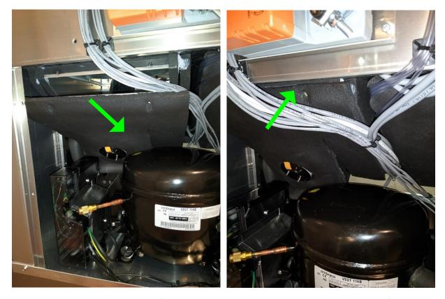
Insert the included UV into the duct opening (using the same method as removing the original panel). NOTE: The UV lamp should NOT be installed yet.
