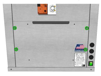
Using the 1/4" driver, remove the four hex-head screws for the lower sheet metal access panel, highlighted in green. Slide out the panel, and set aside. If a CERV2 I/O Expansion board is located on this panel make notes about wire connections and then disconnect any wires to make removing panel possible.
