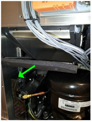
Pull down on the top of the access panel (hinging at the bottom), until the access panel pivots past the wire harnesses. Before removing, take note of how the access panel fits into the metal duct housing, as the new panel will insert the same way. Pull the access panel straight out of the unit, and set aside.
