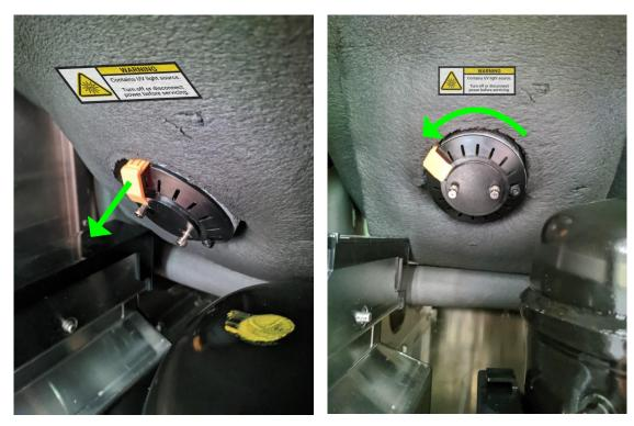
Slightly pull the orange tab for the UV lamp socket, and then rotate the mount counter-clockwise (approx 30 deg.)
