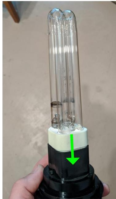
**DO NOT TOUCH THE LAMP GLASS WITH YOUR FINGERS.** Holding the UV lamp by the white plastic base, insert into the UV mount, aligning the four metal pins with the matching holes.
