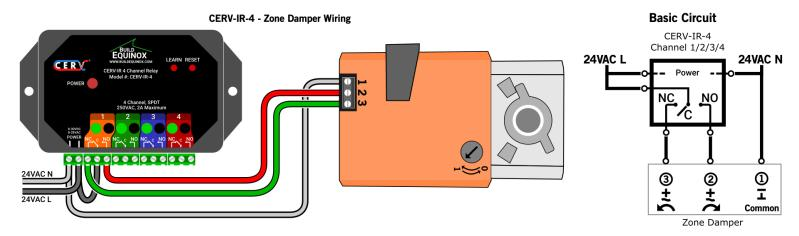
Note: Always confirm zone damper rotation after installation. Rotation direction may be switched with circular 0-1 switch on damper motor.
