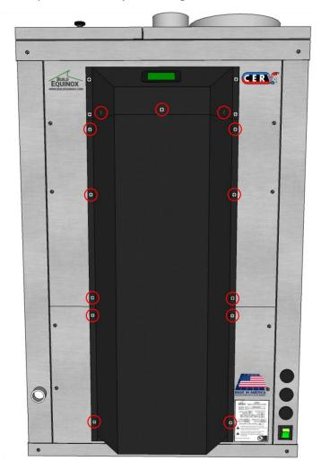
Once the lower front cover is off, the four screws for the lower access panel can be removed. Screw locations are shown below. With the screws removed, the panel will be free to come out. **Note:** If using the I/O Expansion Board, the module will be accessible on this panel. Wiring should be run through the knockout holes and panel slot for the I/O Expansion Board.
