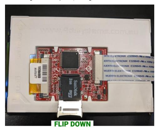
**Step 6:** Remove the SD card, and replace with the new SD card.
