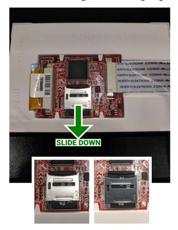
**Step 5:** The metal SD Card housing should now flip down, allowing access to the SD card.
