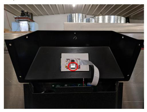
**Step 4:** While lightly pressing on the metal SD card housing, slide it down using a fingernail.
