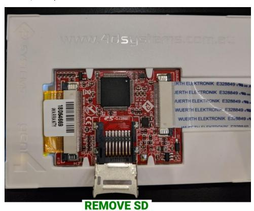
**Step 7:** Follow all previous steps in reverse to re-latch the SD card and reassemble the top touchscreen enclosure. Power may be turned back on after it has been assembled.
