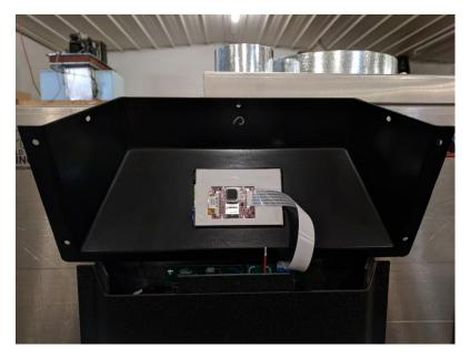
Rotate the top enclosure to see the circuit board on the underside (rotate the bottom towards you, top away from you). A ribbon cable connects the touchscreen to the main control board, and should be left in place. Take care not to bend or dislodge the ribbon cable from its connectors. The MicroSD card is located on the back of the screen held in place by a silver metal clip shown circled in red below.
