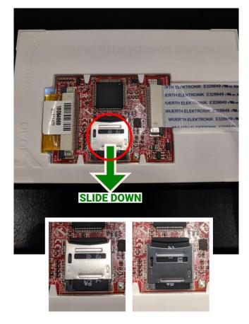
While lightly pressing on the metal SD card housing, slide it down using a fingernail.
