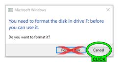
Make sure a Windows computer is being used, a Mac formats the SD card incorrectly and damages the memory card. Once the MicroSD card is inserted into the computer, it may display a warning as shown above. Ignore this warning by clicking the Cancel button.
