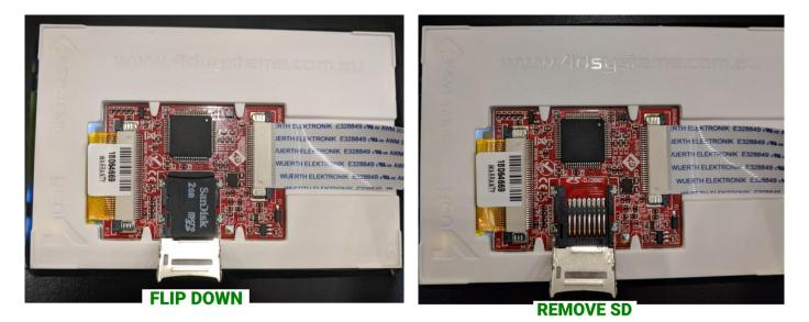
The metal SD Card housing should now flip down, allowing access to the MicroSD card.
