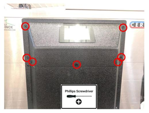
Locate the 7 black phillips head screws mounting the top touchscreen enclosure to the unit (shown below). Remove the screws.
