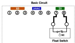
When safety switch is OK (no water), Switch is CLOSED When safety switch faults, Switch is OPEN, system shuts down
